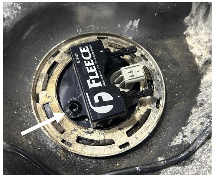
**STEP 14:** Place the fuel tank back under the truck and lift it about six to eight inches below its normal position. Reconnect the fuel lines and the harness connection. If the vehicle is equipped with a fuel transfer tank, connect the transfer fuel line to the port installed in step 13.
