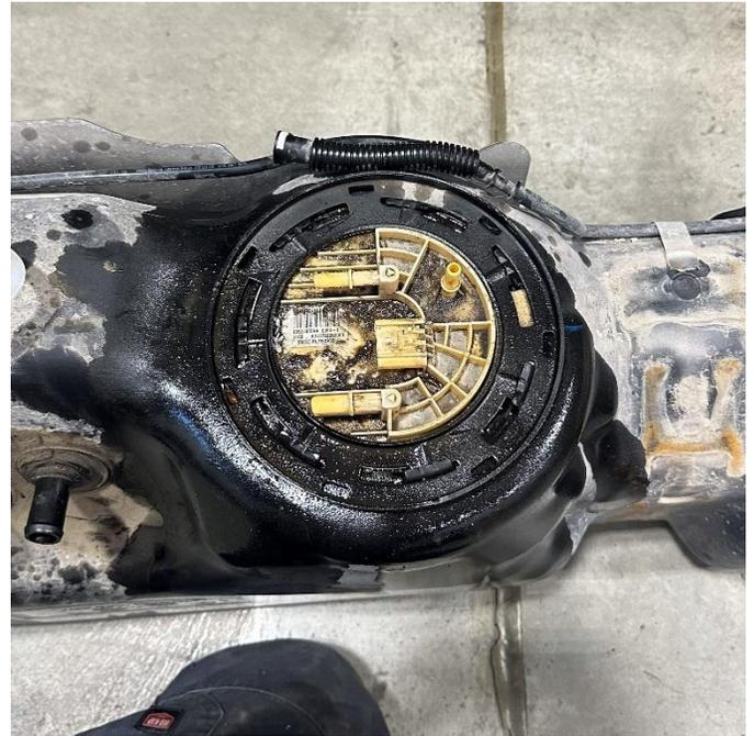
**STEP 24:** Install the included float arm onto the PowerFlo lift pump by carefully clipping the arm into the resistor card as shown at right
