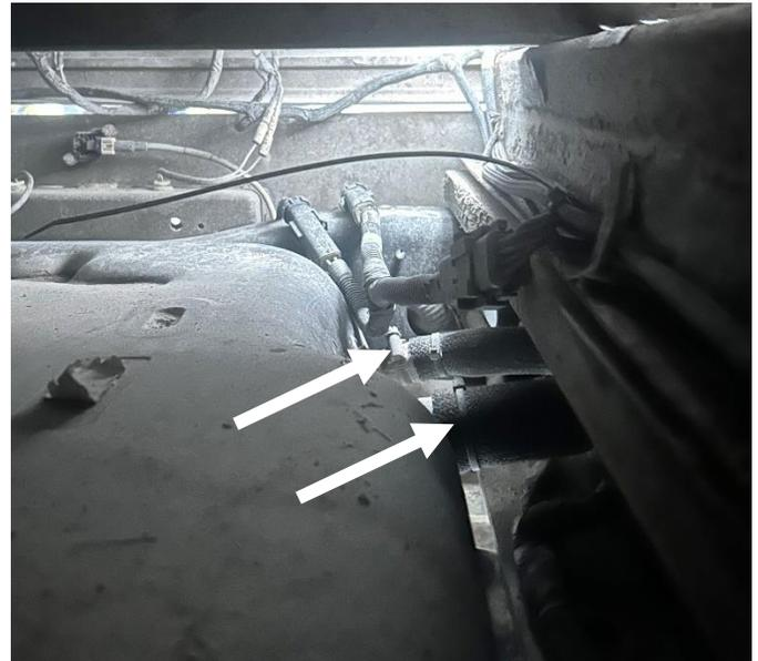
**STEP 4:** Place a floor jack or transmission jack underneath the fuel tank. Remove the 8 bolts retaining the saddle tank using a 16mm socket or wrench. There are four bolts on the front and four bolts on the rear of the tray retaining the tank.
