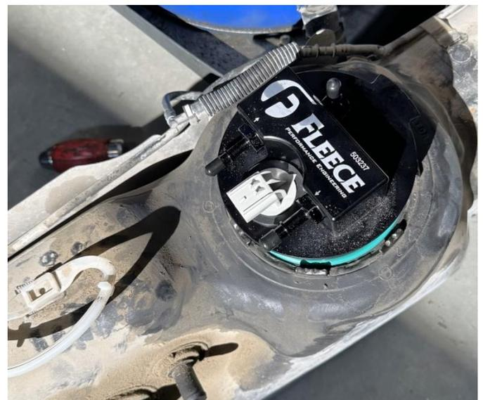
**STEP 26:** Lift the tank about five to six inches below its installed height and reconnect all fuel lines and the electrical connector.
